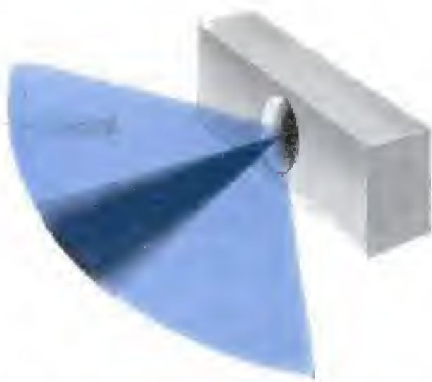
Speaker tends to beam high-frequency sounds straight out in narrow band. Bass sounds spread more evenly
